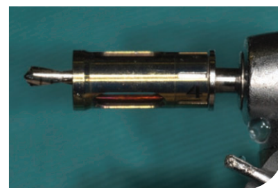
∅ 2.2 twist drill with 4.0 mm stopper
